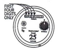
Occasionally you need to read your water meter. If you have a basement, that is where it will be. Pictured is a sample of the water meter. Just read the four digits as shown on the drawing.
